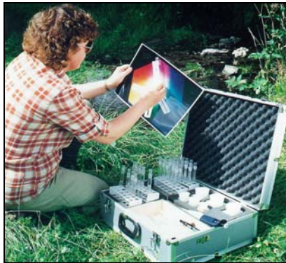
Fig. 1. Field analysis of stream water for Cu by colorimetry using visual comparison with a universal colour chart (from British Geological Survey flyer, Analytical Geochemistry Group, Capability Profile).
